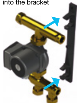
Figure 17: Clip the control pack into the bracket
