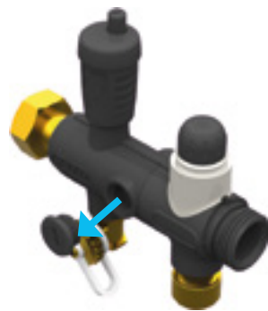
Figure 9: Remove plugs on return arm
