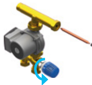
Figure 14: Loosen the connection
