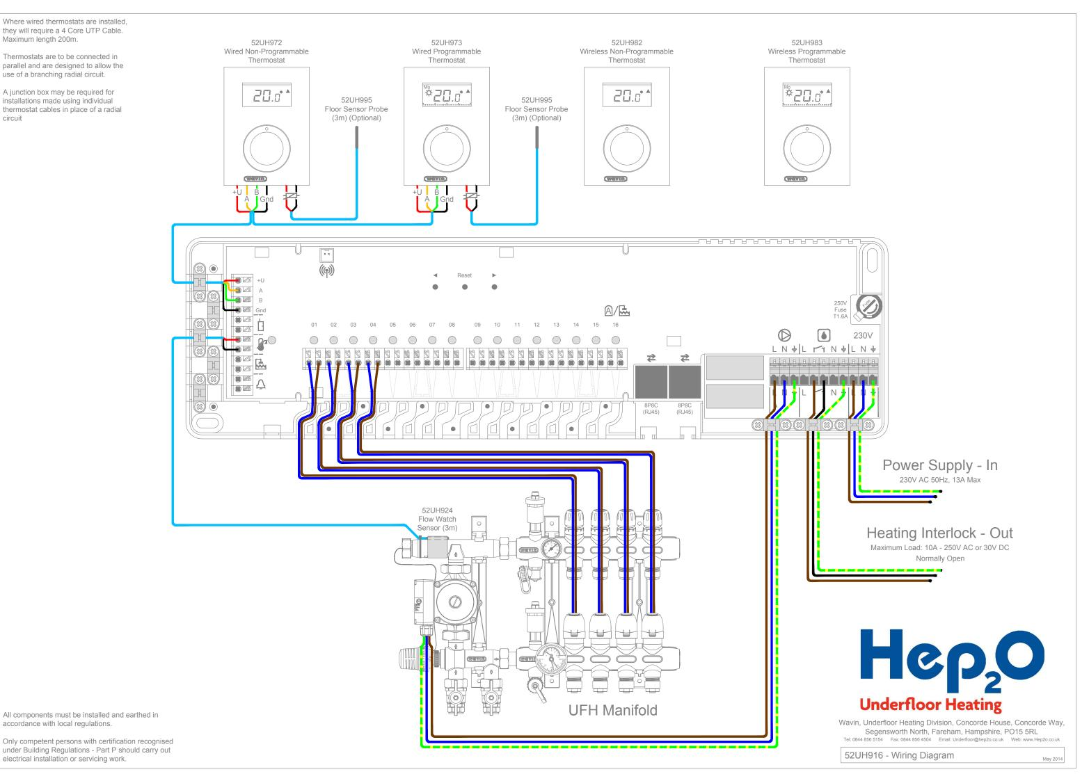
Where wired thermostats are installed, they will require a 4 Core UTP Cable. Maximum length 200m.
