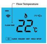
When the neoStat is set to use both the air & the floor sensor, the room temperature will be displayed by default.
