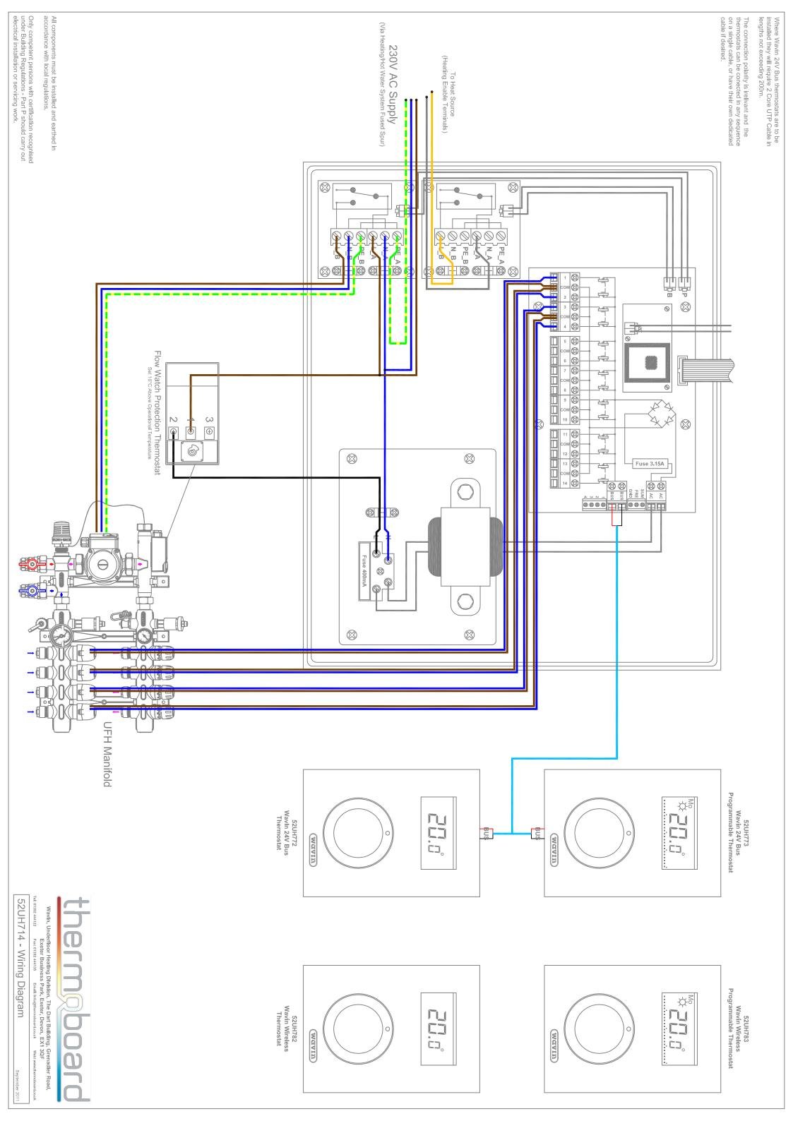
An automatic bypass valve should be provided in conjunction with any requirements for a minimum pipe length specified in the boiler manufacturer's instruction. The connection polarity is irelivant and the thermostats can be conected in any sequence on a single cable, or have their own dedicated cable if desired. Where Wavin 24V Bus thermostats are to be installed they will require 2 Core UTP Cable in lengths not exceeding 200m. Return
